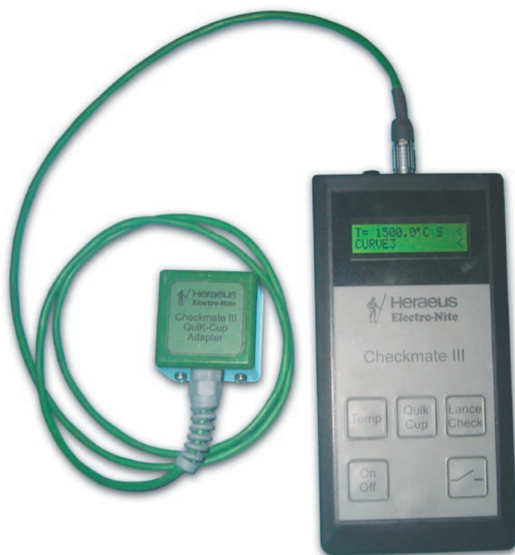
Fig. 20 – Checkmate Positherm/Quik-Cup with QC adapter
