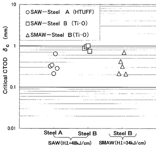
Fig. 3 CTOD test results of welded joints
