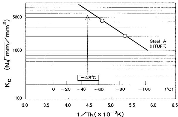
Fig. 2 Center deep notch test results of SAW welded joints
