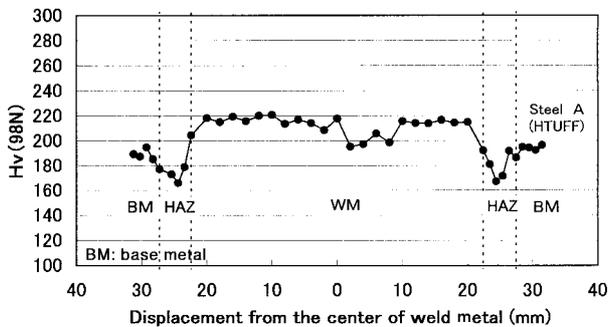
Fig. 4 Hardness distribution of SAW welded joints
