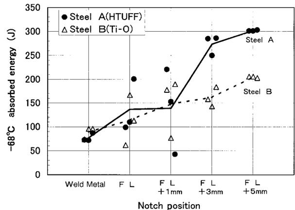
Fig. 1 Charpy impact test results of SAW welded joints
