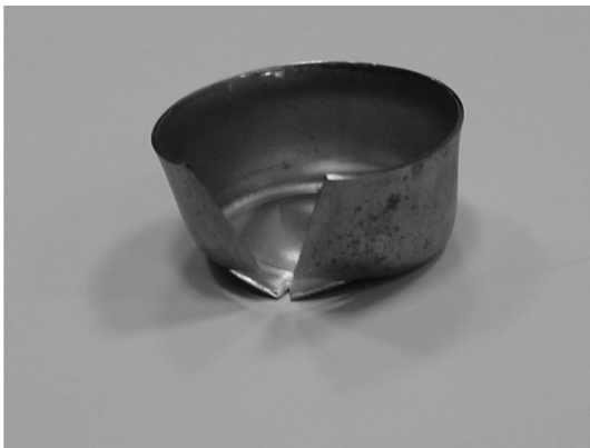
图 9 DBTT 试验开裂试样 Fig. 9 DBTT test sample
