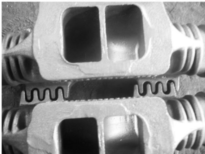
图 9 铸件无缩松 Fig.9 Casting without shrinkage porosity
