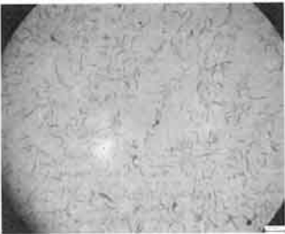
图4 2#试样石墨组织 Fig.4 Graphite structure of 2# sample
