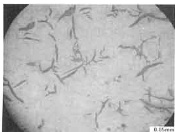
图6 2#试样基体组织 Fig.6 Matrix structure of 2# sample
