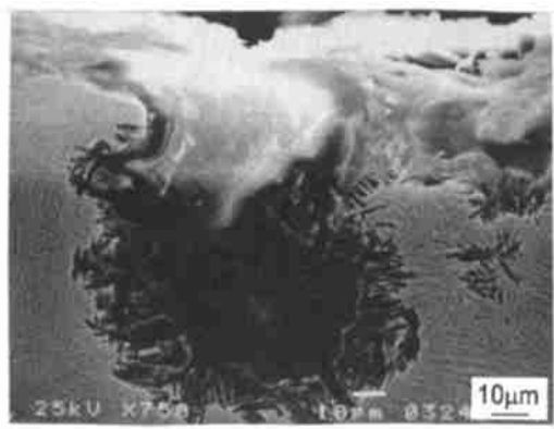
Fig.3 SEM of corrosion pit
