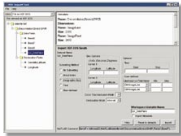
HDF data from a satellite, selected and imported into MATLAB using the MATLAB HDF Import Tool.
